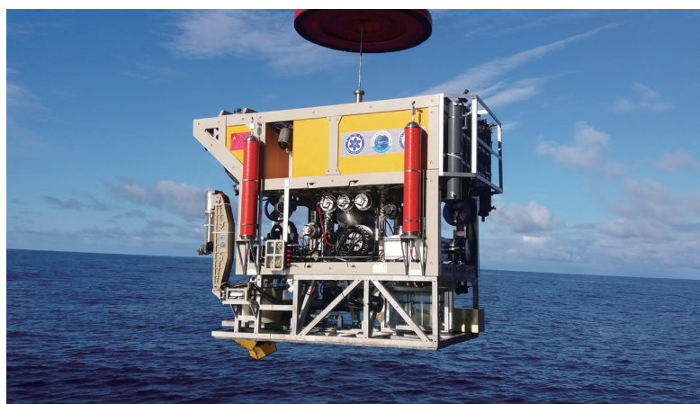
图2 “海星 6000”水下遥控航行器 Figure 2 “Haixing 6000” remotely operated vehicle
